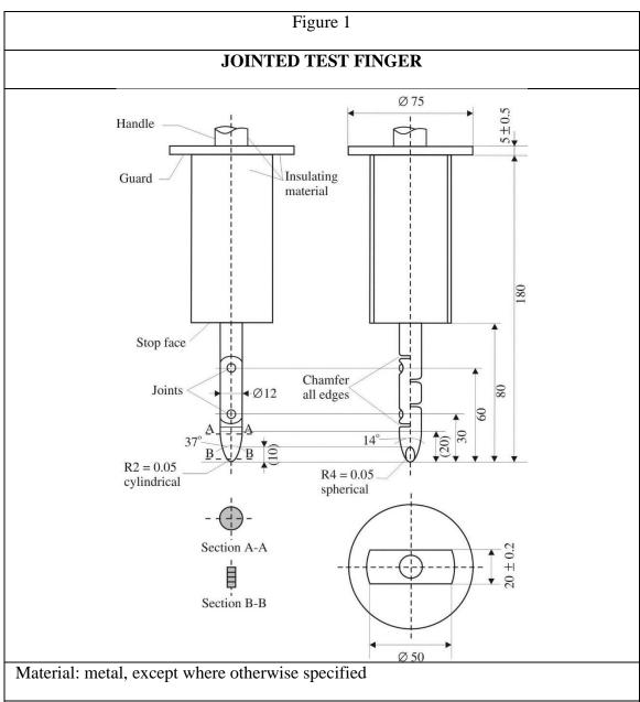
Linear dimensions in millimeters
